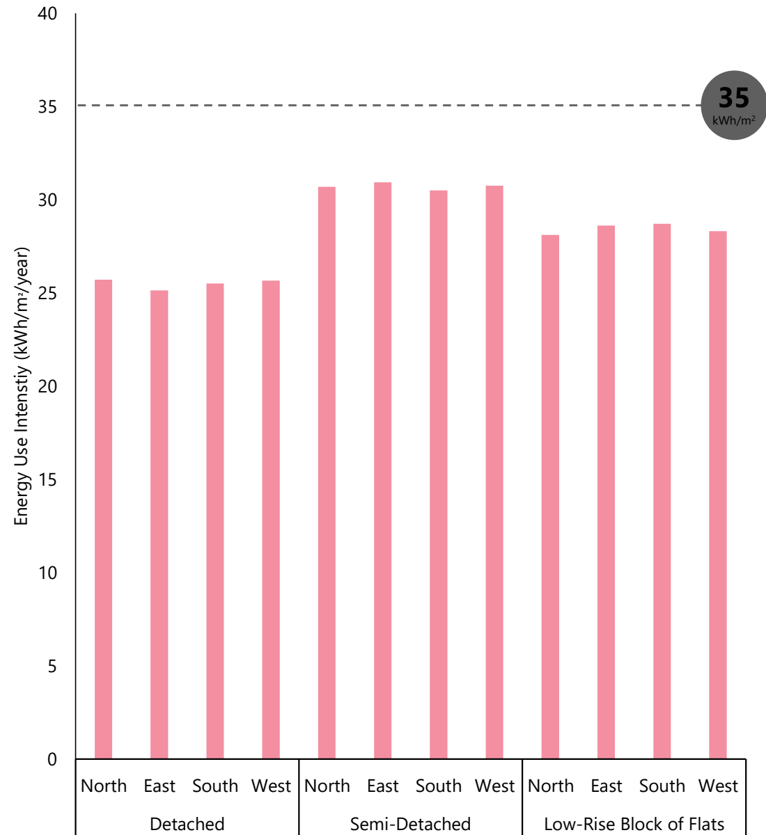
Figure 8.2: Energy use intensity results from PHPP modelling of all the domestic typologies at different orientations
