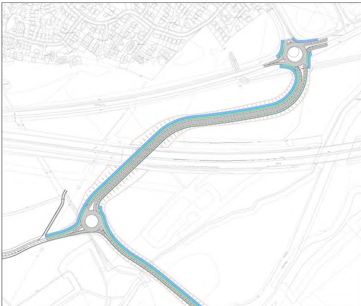
Figure 10 New access to Lower Earley Way landing at the B3270/Meldreth Way Roundabout (source: Abley Letchford Partnership Consulting Engineers, drawing no. A392-097)
