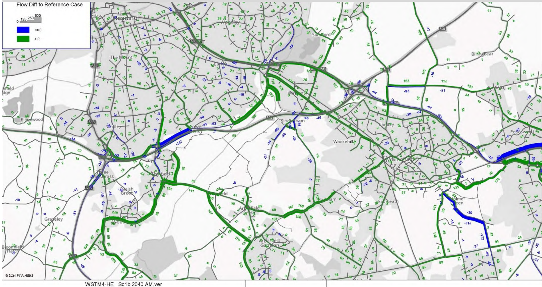
Figure 31 Actual Flow Differences. 2040 Scenario 1B 'Hall Farm' minus Ref Case. AM Peak
