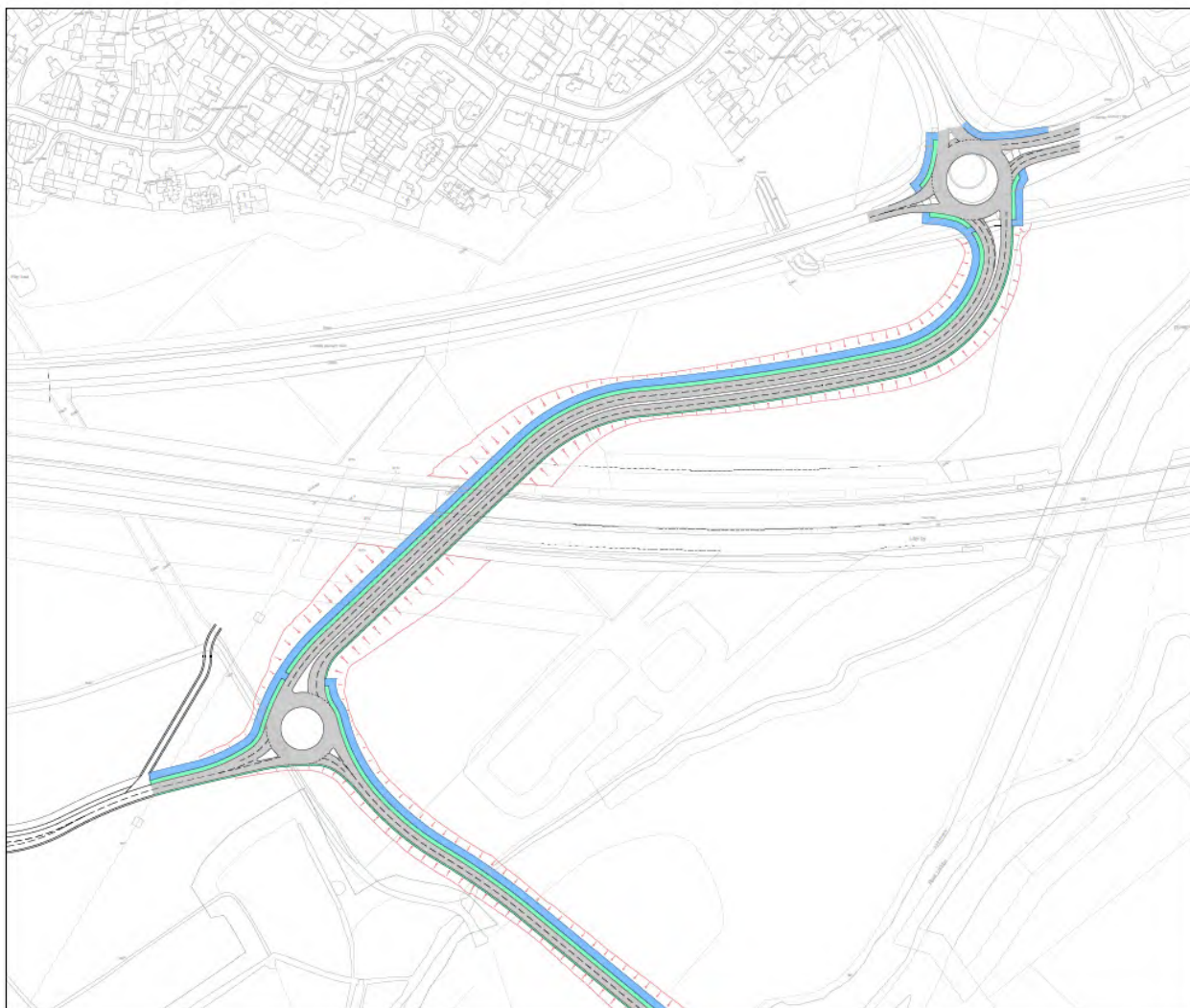
Figure 26: New access to Lower Earley Way landing at the B3270/Meldreth Way Roundabout (source: Abley Letchford Partnership Consulting Engineers, drawing no. A392-097)
